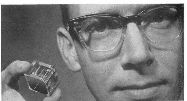
SPECIAL PROJECT, conducted by TDP student Dean E. in a volume less than one cubic inch. Tiny prototype Gladow (7224), produced 1000-to-one power-reduction unit used five Mylar belt stages instead of gears.
